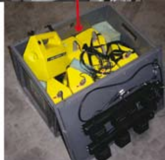
MITRALUX L140 rechargeable lights, integrated into the light trailer for civil defence vehicles. With special transport and charger box.
